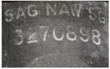
Those of us who are old enough to remember "Print Shop" in high school will recall the difficulty in handling the small pieces of type-face, and clamping them into dies. Note also that two different fonts were used in the marking of these two receivers. The letters S, G, N, and W are all slightly different.
