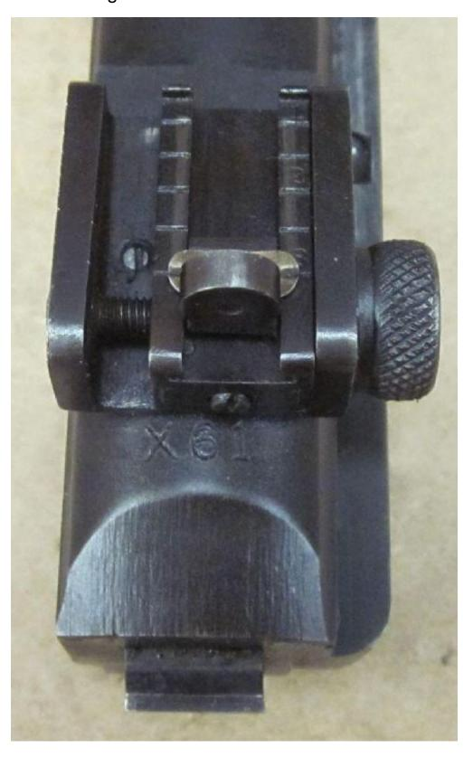
The small shallow screw (shown closeup below) secures the sight to the dovetail. When screwed down tight, it exerts uplift pressure on the sight against the dovetail. Think of it as a type of staking. But, look closely at
