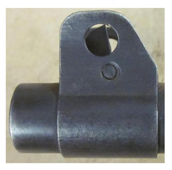
The T21 adjustable rear sight sits in a very shallow dovetail on a rather flat-topped receiver. Compare this profile to that of a standard M1 Carbine. The receiver construction characteristics confirm manufacture of this receiver in late 1942. (See Carbine Club newsletter 346-2 article by Chris Albright.)
