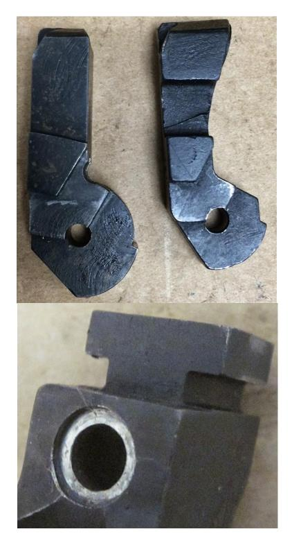
In the photo above, note that the recess in the trigger housing to seat the hammer spring and plunger was modified after the black oxide (dull blue) finish was applied. Major Eli Cooper had a degree in Mechanical Engineering. During WWII, he rose to the position of Head of Production Design and Development, R&D Division of the Ordnance Department. He received postwar patents for the M15 Grenade Launching Sight (for the Carbine and M1 Garand, a patent he shared with John C. Garand),
